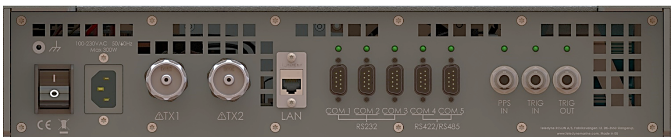
Figure 4: DESO 5DS rear panel cable connections
